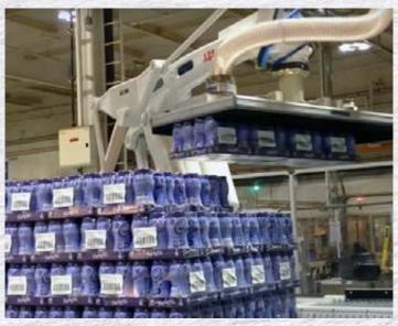
Palletizing of boxes, trays and shrink wraps can be enabled with the same UniGripper. Depending on product properties as well as what is most optimal for each installation, the vacuum source can either be venture ejectors or a side channel blower.
