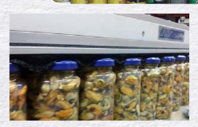
Each Unigripper is customized according to sizes of current and future products. All parts from valve design to source for vacuum generation are optimized to make an energy efficient and versatile solution.
